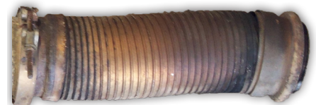
Leaky flex connector
